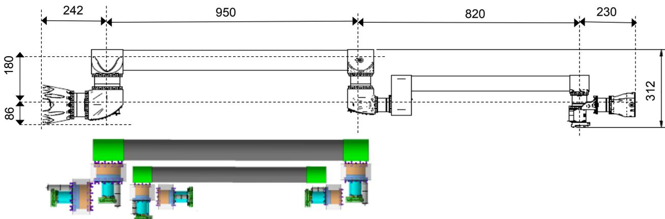
Figure 2. LARAD kinematic design, deployed (top) and stowed (bottom) configuration
