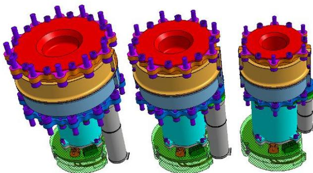
Figure 8. Modular Actuation Cores (MACs), resulting joint designs
