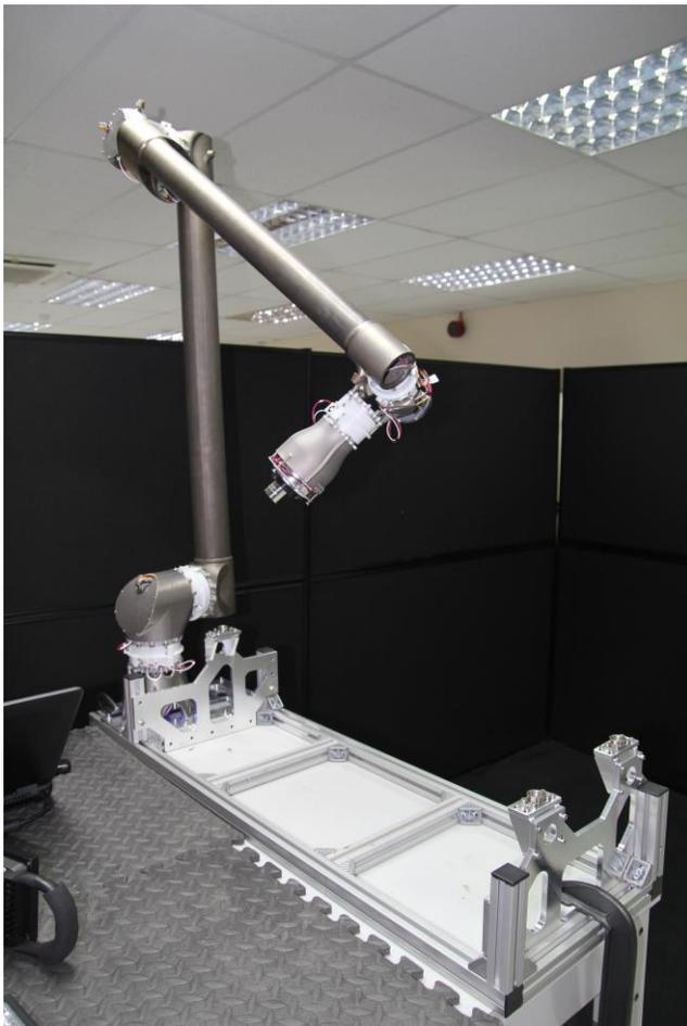
*Figure 15. LARAD fully assembled hardware*
