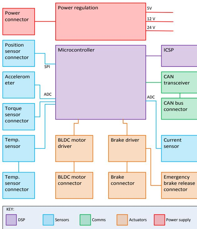
Figure 13. Architecture design for control electronics
