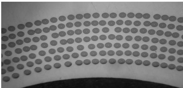
Figure 6. TiSiC metallic composite transverse cut, SiC fibers (dark grey) embedded in a Ti matrix (light grey)
