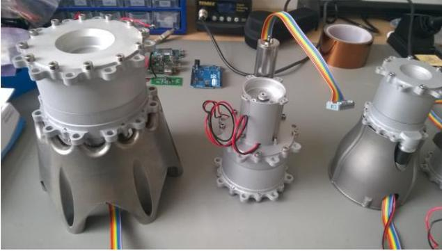
Figure 11. Integrated MACs (w/o electronics) with some ALM parts, large (left), medium (centre), small (right)
