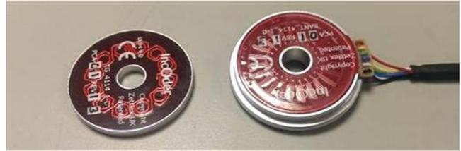
Figure 10. View of the Zettlex position sensor prototype, rotor (left), stator (right)
