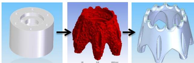
Figure 3 ALM topology optimisation process; interface and volume definition (left), superimposed load paths (centre), resulting final part (right)
